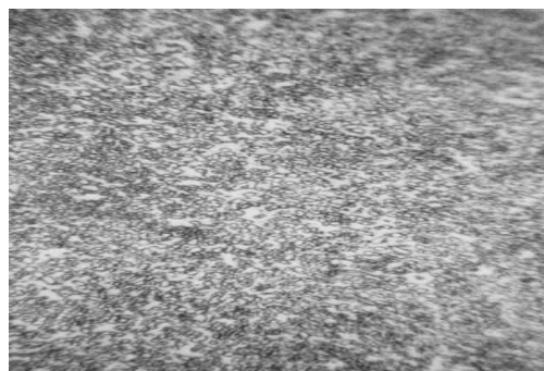
Fig. 5. Optical micrograph of 100Cr6 steel after spheroidising annealing (Condition A), 800x. Ferritic matrix with uniformly distributed globular cementite carbides. Nital etch.
