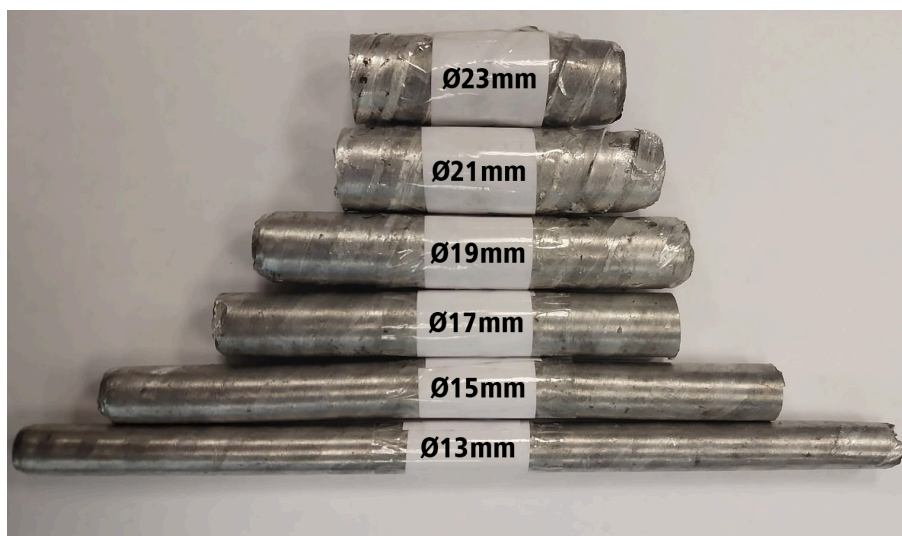
Fig. 3. Final aluminum rolling samples for the various stages of defect formation.
