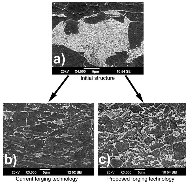
Fig. 2. Microstructure of DIN 1.2542 steel.
