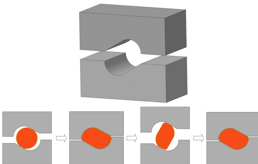
Fig. 1. Tool construction and broaching scheme in a new design forging tool.
