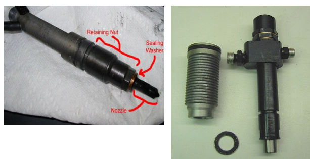
Fig. 3. Photographs of the primary fuel injector (a), a pilot fuel injector (b).
