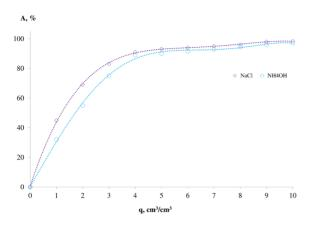
Fig. 7. Dependence of the degree of desorption of nitrates from Dowex Marathon WBA anionite in  $PO_4^{3-}$  form on the passed volume of regeneration solutions.
