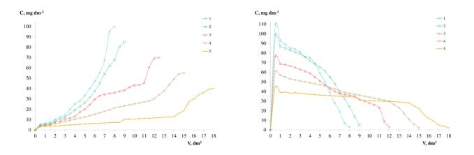
Fig. 5. Dependence of the initial concentration of phosphates (a) and chlorides (b) on the passed volume of sodium phosphate solution with a concentration of 100 (1), 85 (2), 70 (3), 55 (4), 40 (5) mg-eq dm<sup>-3</sup> through the low basic anionite DOWEX MARATHON WBA in chloride form.
