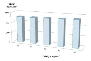
Fig. 6. Dependence of total dynamic exchange capacity (TDEC) from Dowex Marathon WBA anionite on their concentration anions the solution.
