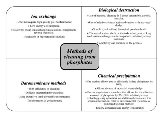
Fig. 1. Advantages and disadvantages of the methods used to remove phosphates from water.
