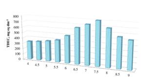
Fig. 3. Dependence of TDEC on pH on the passed volume of sodium phosphate solution with a concentration of 100 mg-eq dm<sup>-3</sup> through the low basic anionite DOWEX MARATHON WBA in chloride form.
