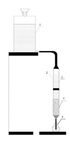
Fig. 2. Ion-exchange experimental installation filled with DOWEX MARATHON WBA ion-exchange resin: 1 container with water containing phosphates; 2 - a column with a diameter of 19 - 30 mm; 3 - a layer of water, above the ionite; 4 - layer of ionite DOWEX MARATHON WBA; 5 - a flask for collecting purified water after filtering through ionite.
