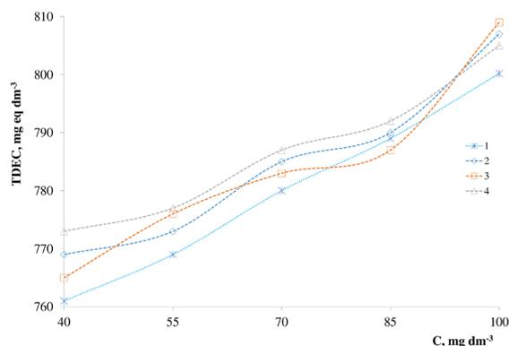
Fig. 4. Dependence of TDEC on temperature on the passed volume of sodium phosphate solution with a concentration of 100 mg-eq dm<sup>-3</sup> through the low basic anionite DOWEX MARATHON WBA in chloride form: 1 - 10°C; 2 - 20°C; 3 - 30°C; 4 - 40°C.
