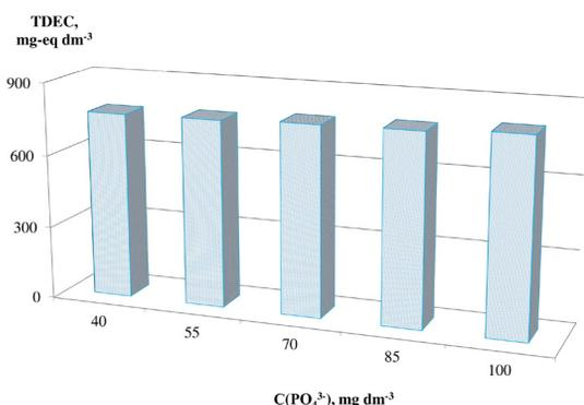
Fig. 6. Dependence of total dynamic exchange capacity (TDEC) from Dowex Marathon WBA anionite on their concentration anions the solution.
