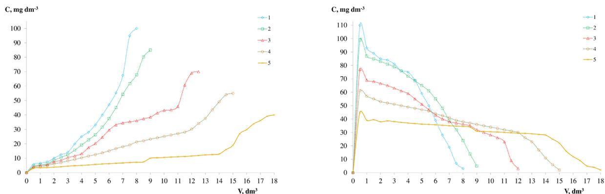
Fig. 5. Dependence of the initial concentration of phosphates (a) and chlorides (b) on the passed volume of sodium phosphate solution with a concentration of 100 (1), 85 (2), 70 (3), 55 (4), 40 (5) mg-eq dm<sup>-3</sup> through the low basic anionite DOWEX MARATHON WBA in chloride form.
