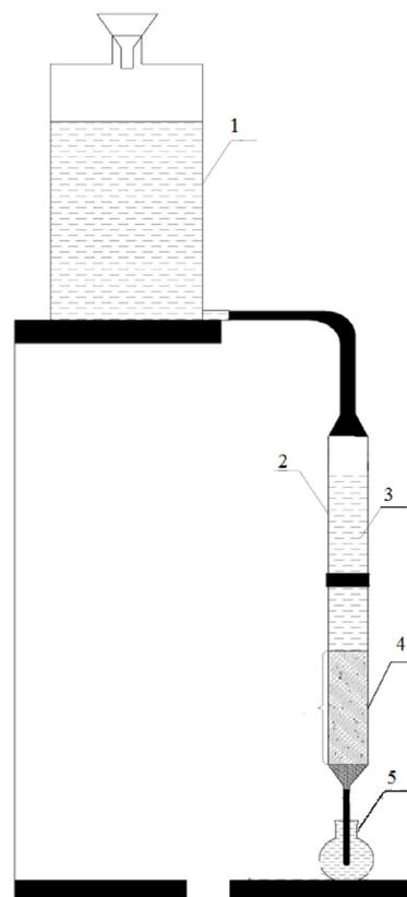
Fig. 2. Ion-exchange experimental installation filled with DOWEX MARATHON WBA ion-exchange resin: 1 - container with water containing phosphates; 2 - a column with a diameter of 19 - 30 mm; 3 - a layer of water, above the ionite; 4 - layer of ionite DOWEX MARATHON WBA; 5 - a flask for collecting purified water after filtering through ionite.
