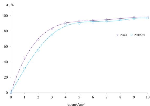
Fig. 7. Dependence of the degree of desorption of nitrates from Dowex Marathon WBA anionite in  $\text{PO}_4^{3-}$  form on the passed volume of regeneration solutions.
