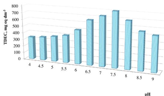
Fig. 3. Dependence of TDEC on pH on the passed volume of sodium phosphate solution with a concentration of 100 mg-eq dm<sup>-3</sup> through the low basic anionite DOWEX MARATHON WBA in chloride form.
