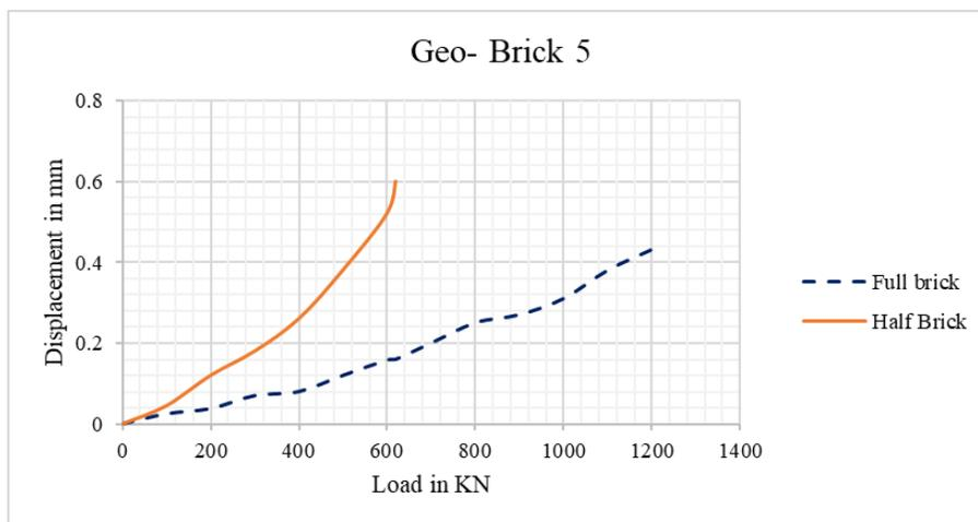
Fig. 10. Displacement vs. load in the GBFS-FA geopolymer prism.
