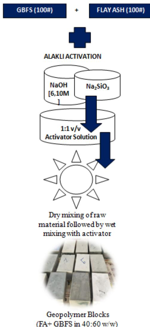
Fig.2. Schematic of process steps for geopolymer development.
