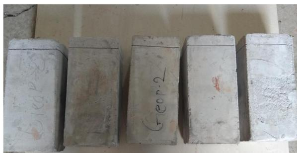
Fig. 4. Geo-brick from FA and GBFS combination.
