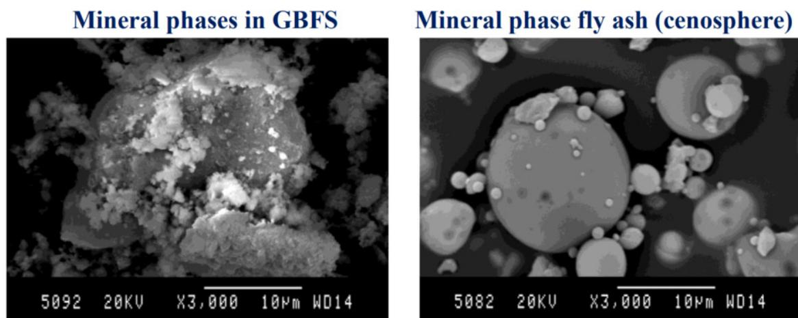
Fig. 3. Mineral phases in GBFS and FA using SEM.
