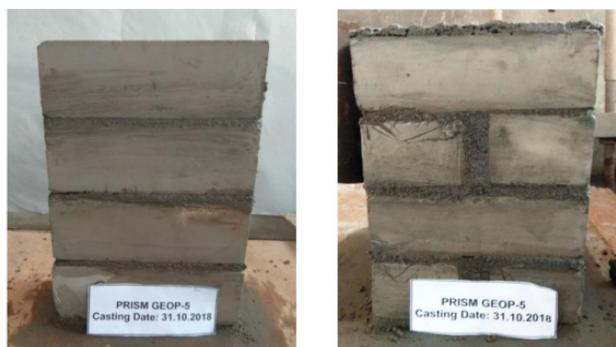
Fig. 8. Single and double brick geopolymer prism.
