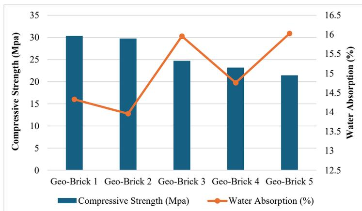
Fig. 5. Compressive strength and water absorption test results for Geo-Bricks.
