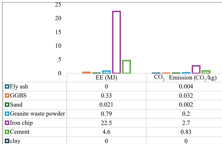
Fig. 1. Embodied energy and CO<sub>2</sub> emissions for raw precursors used in geopolymer [13].
