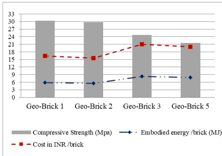
Fig. 11. Compressive Strength, Embodied Energy and Cost per geo-brick.
