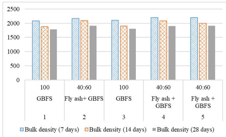
Fig. 6. Density, kg m<sup>-3</sup> variation with different proportion.
