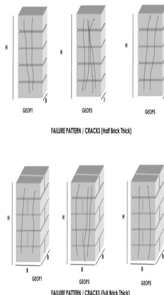
Fig. 9. Crack patten observed in the GBFS-FA geopolymer prism.
