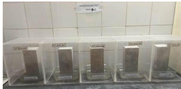
Fig. 7. Efflorescence test on Geo-Brick samples.
