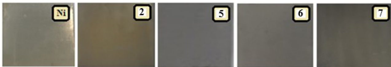
Fig. 4. Photographic images of coatings of Ni (the first photo) and of SnNi(C) on copper electrode (samples „2“, „5“, „6“ and „7“ from Table 1).
