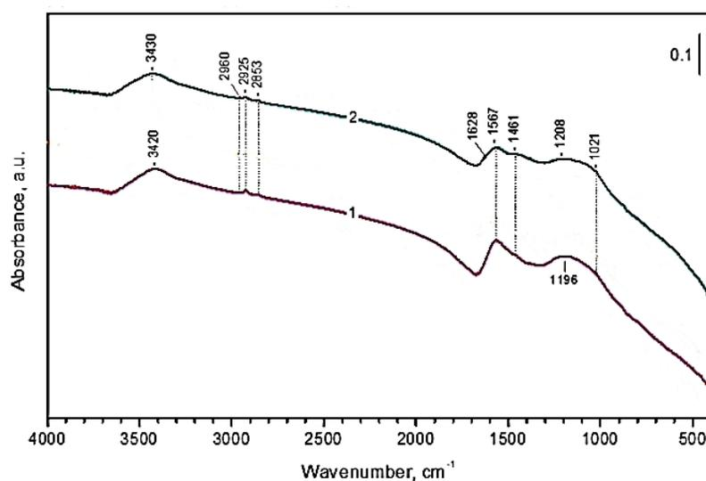
Fig. 4. FT-IR spectra of the activated samples 1 - ACK1, 2 - ACK2.
