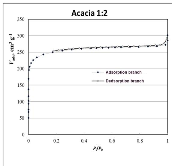
Fig. 3. Low-temperature nitrogen adsorption isotherm at 77.4 K of ACK2.
