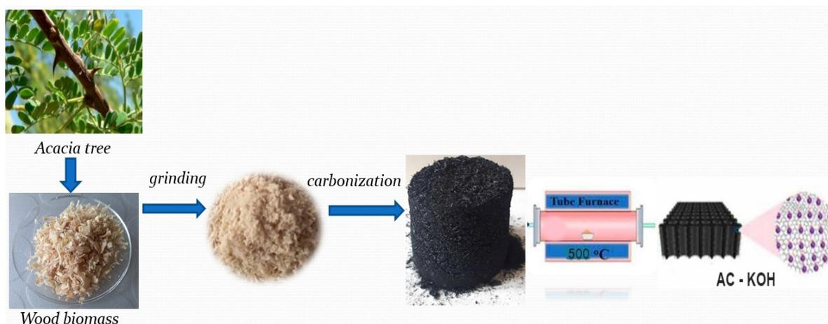
Fig. 1. Process of the production of AC based on acacia wood biomass.
