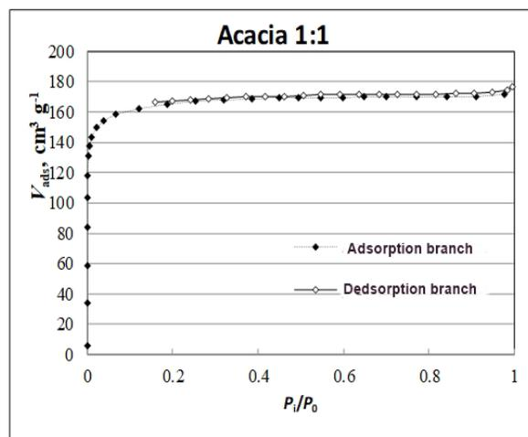
Fig. 2. Low-temperature nitrogen adsorption isotherm at 77.4 K of ACK1.
