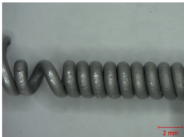
Fig. 8. Wire winding test Ø 1 mm from MC10 alloy.
