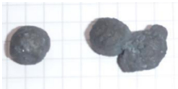
Fig. 6. Pellets after reduction in rotary kiln.
