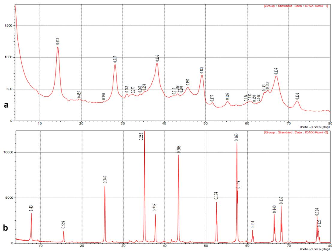
Fig. 2. X - ray diffraction patterns of the initial (a) and calcined (b) high-alumina waste from the ShGCC.
