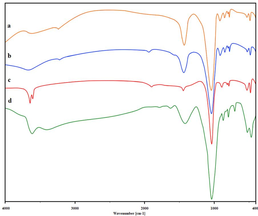
Fig. 3. IR spectrum curves of kaolin grade AKF - 78 (a), AKS - 30 (b), Alliance (c), Kasan bentonite (d).
