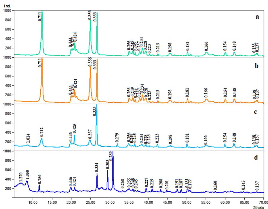
Fig. 1. X - ray diffraction patterns of clay raw materials where: (a) kaolin grade AKF - 78; (b) AKS - 30; (c) Alliance kaolin; (d) Kasan bentonite.
