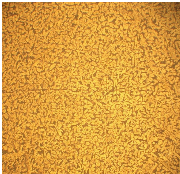
Fig. 2. Base alloy microstructure CuAl9Fe3 ( \times 63 ) [4].
