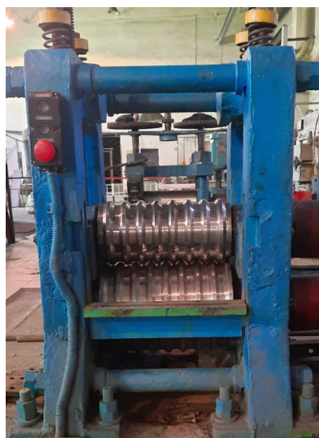
Fig. 2. Cage with relief rolls of different diameters.
